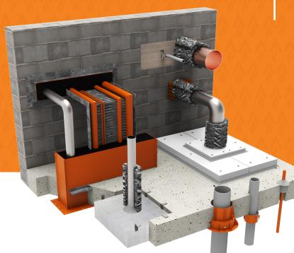
Service Penetrations requiring three or four hour FRL's often have very limited solutions available if any at all. Trafalgar Fire has a wide range of systems that have been specifically fire tested for this application to cover a large range of service types to meet the high performance required.
